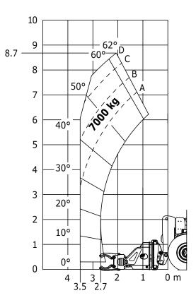
Machine on tyres with CH10 2 tons (Norm AS1418.19)
