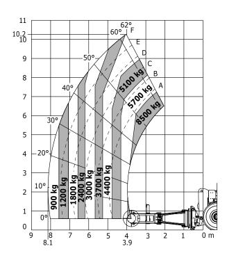
Machine on tyres with CH4-1,2 tons (Norm AS1418.19)
