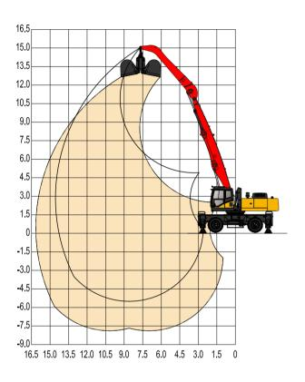
Movable boom 8.6m, loading stick 6m, Hinge point at the top point
